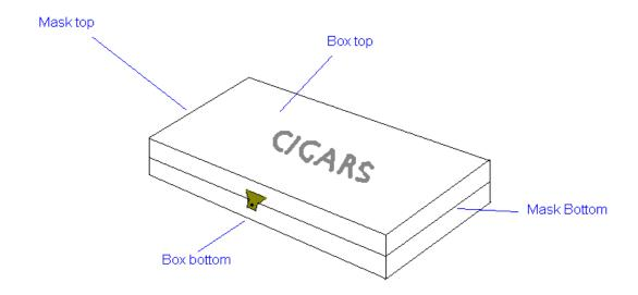
2. Near the mask bottom cut a) a 2-3 inch circular hole on the box top for mounting the diaphragm and b) a mouth-shaped sound hole on the box bottom.
